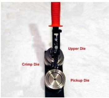
**Step 5:** With the magnet back still in the Crimp Die pull the handle a second time.
