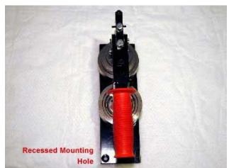
**Step 3:** Pull the handle down, easily crimping the shell, graphic, and mylar in the Upper Die.
