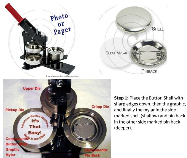
**Step 2:** Rotate the part of the machine that has the button shell, graphic, and mylar clockwise until it is underneath the Upper Die.
