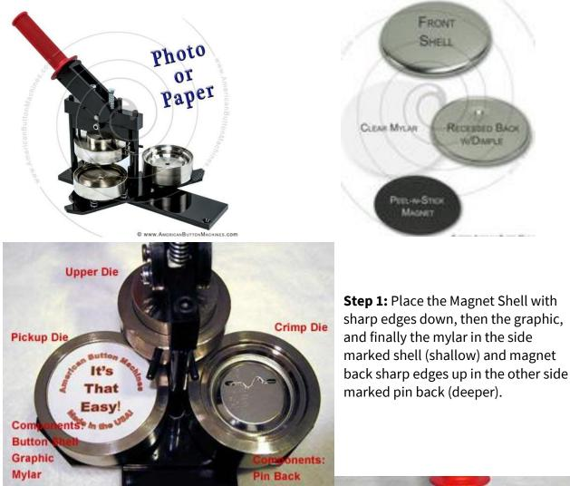
**Step 2:** Rotate the part of the machine that has the Magnet shell, graphic, and mylar clockwise until it is underneath the Upper Die.
