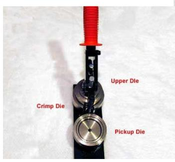
**Step 5:** With the pin back still in the Crimp Die pull the handle a second time.
